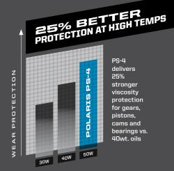
WHY VISCOSITY MATTERS: Polaris engines are designed to operate using oils rated at a specific viscosity. Viscosity is the measure of an oil's resistance to flow and shear and a way to gauge an oil's "film strength", which is a critical component in preserving engine life when an oil is subject to high heat or heavy loads.
