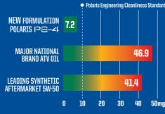
ASTM D6335. In 3rd party against 9 competitive products Polaris PS-4 had less than half the deposits compared to the next closest product. No other tested products met Polaris Engineering standards for deposit cleanliness.
