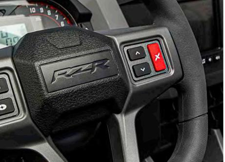
The industry's only steering-wheel-mounted ride adjustment allows you to stay in control when unexpected terrain hits. Instantly attain full-firm suspension settings for one full
